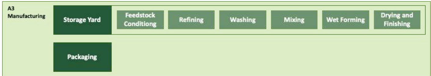
Figure 2. Cellulosic Fiberboard manufacturing process
