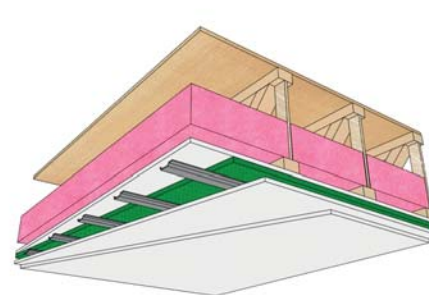
Ceiling with addition STC56 (Estimated value)
