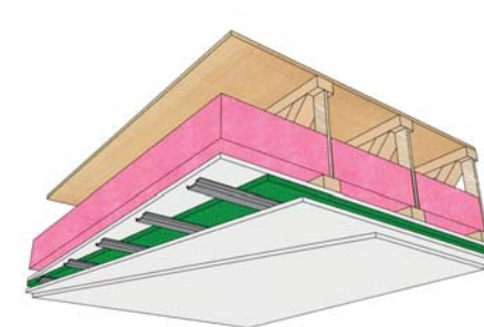
Ceiling with addition STC56 (Estimated value)
